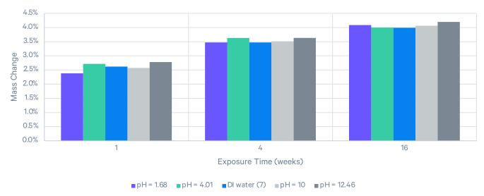
**Treatment Method:** 5 mm by 5 mm by 5 mm cube submerged in solutions at 40  $^{\circ}$  C
