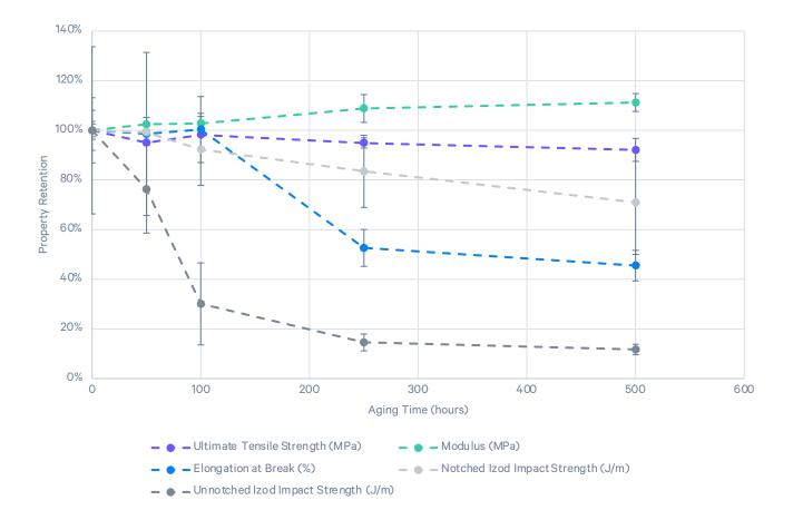
ASTM 4459: Q-Sun XE-1, 0.8 W/m²/nm at 420 nm, 55  $^\circ \rm C$
