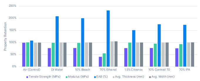
**Treatment Method:** Samples submerged in test liquid for 28 days at 23 °C then removed from test liquid and washed with DI water.
