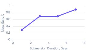
\*\*Distilled Water Mass Gain vs. Submersion Duration
