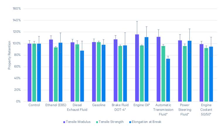
**Treatment Method:** Samples submerged in test liquid for 30 minutes at 23 °C or 50 °C (starred) then removed from test liquid and allowed to sit at ambient room temperature conditions for 1 week (samples were not wiped). **Test Method:** ISO 527-2, Type I, 5 mm/min
