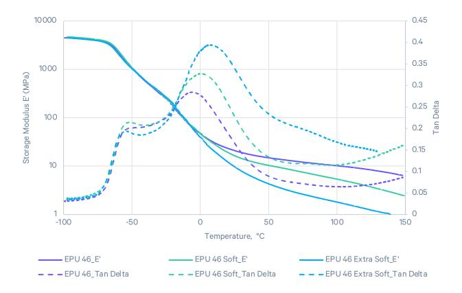
EPU 46 Black Part A and respective Part B options were used to obtain the data Parts were processed using an L series printer and wiped clean. The cleaned parts were baked following the EPU 46 baking schedule Test method: ASTM D4065, 2 °C/min, 1Hz
