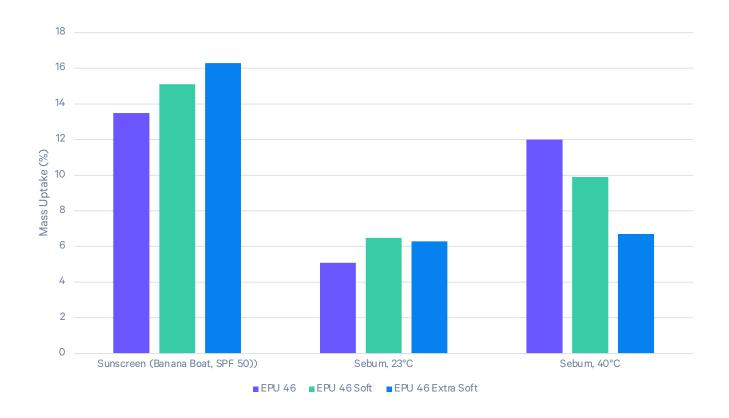
EPU 46 Black Part A and respective Part B options were used to obtain the data Parts were processed using an L series printer and wiped clean. The cleaned parts were baked following the EPU 46 baking schedule
